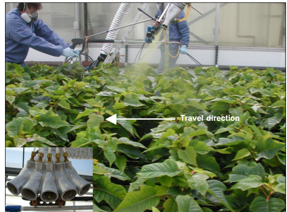
Figure 5. Five-port, air-assist sprayer with XR11003 nozzles.
